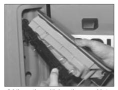
... then withdraw the assembly to the outside of the vehicle
